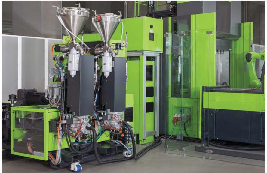
**ENGEL's solution for in-situ polymerisation for the production of fibre-reinforced thermoplastic components is characterised by particularly compact system technology (All pictures: ENGEL)**
