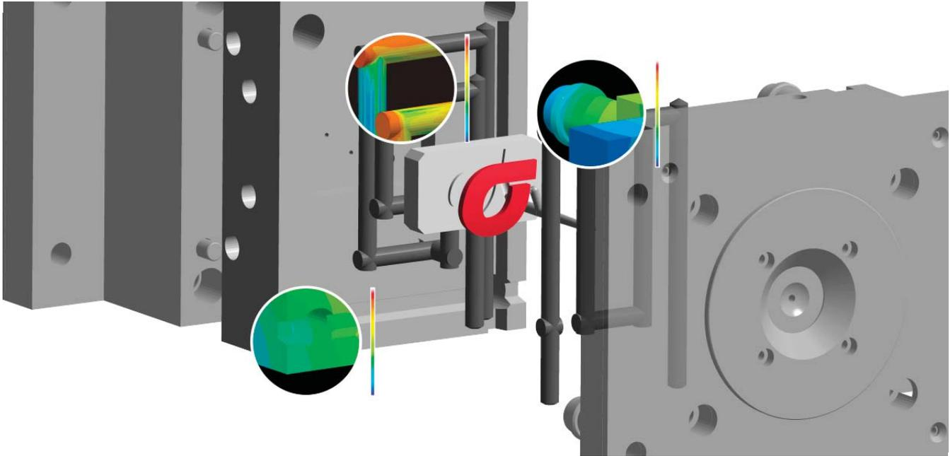
*SIGMASOFT® provides a variety of methods to forecast the shrinkage and warpage of plastic parts. Along with this, one can also simulate the deformation of inserts or core pins during filling. SIGMA simulates and compares the deformation of core pins made of two different mold materials under equal process conditions. The calculations are based on the imbalanced melt flow inside the cavity and the mechanical properties of the two materials.*
