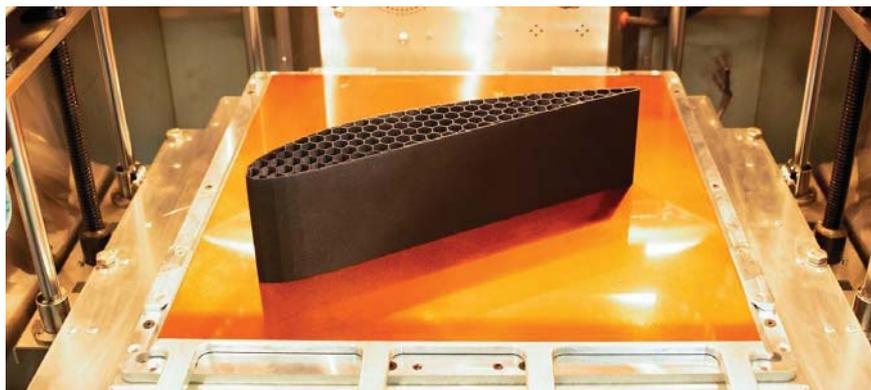
*A part made from Solvay KetaSpire® AM FILAMENT CF10 LS1 – a carbon fiber-loaded PEEK material*
