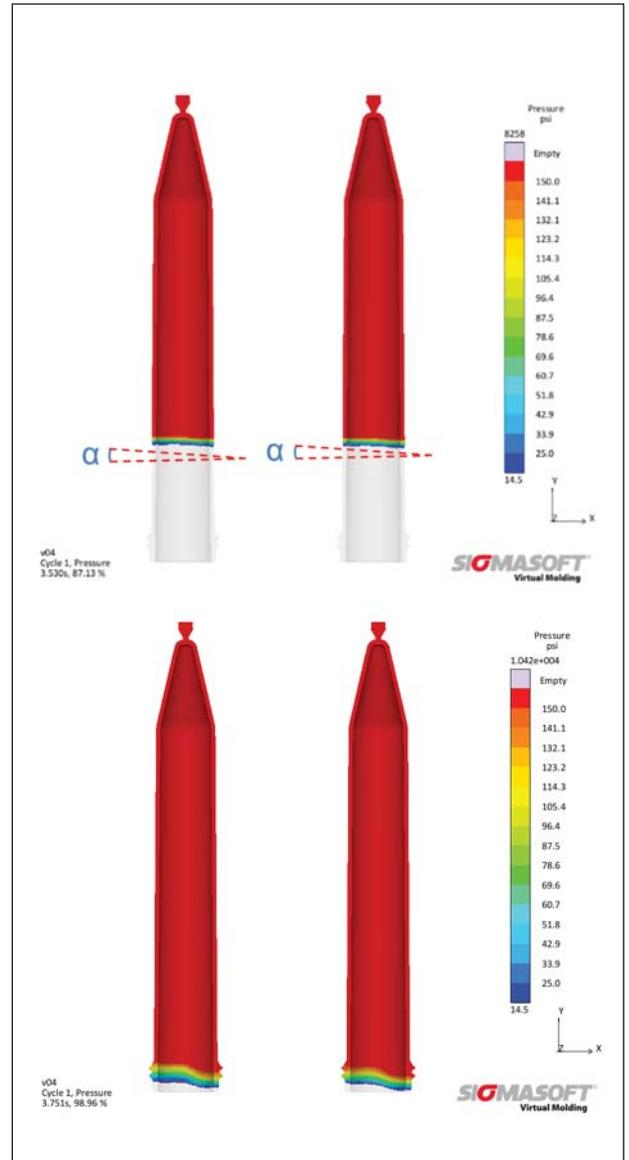
**FIGURE 2** – Demonstration of the melt pressure in two cavities with core pins made of tungsten carbide (left) and 420 stainless steel (right) – The upper section shows the point in filling where the imbalance is visible for the first time. At the end of filling (lower section) this phenomena can be seen clearly
