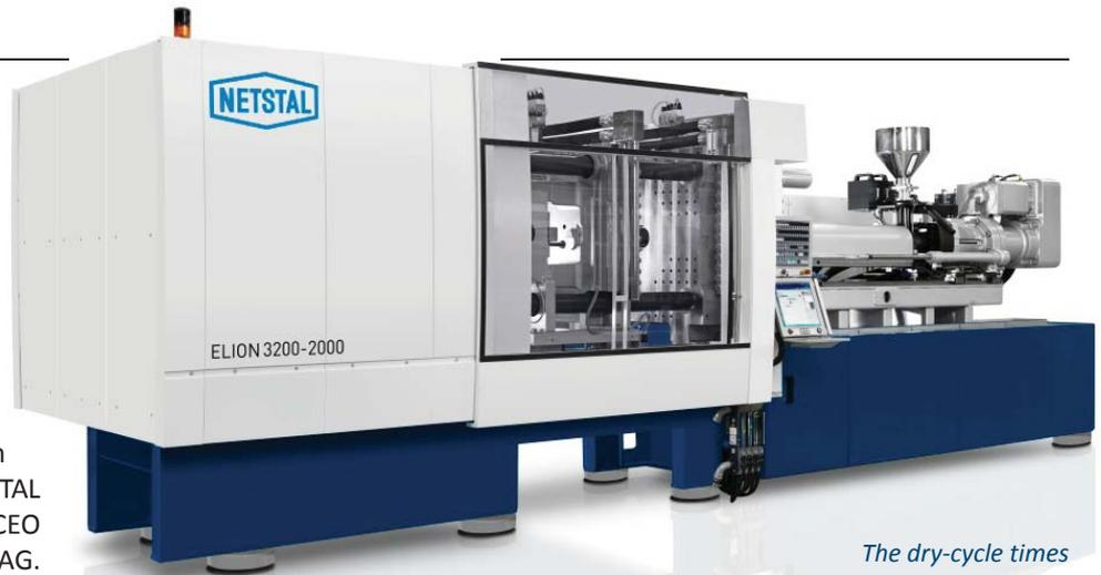
*The dry-cycle times of the proven NETSTAL ELION have been reduced by up to 0.2 seconds across the entire model range*
