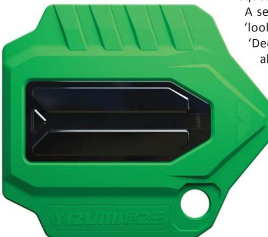
*Engine cover with thermoplastic carrier and second component flooded PU after first trial*
